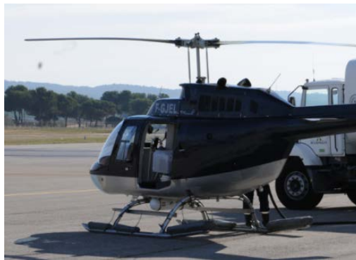
Figure 6 Image showing the PicoSAR mounted on the backseat behind a protective plastic cover and the door removed for less interference.
